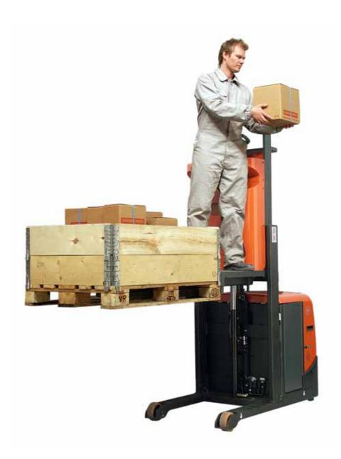
The OSE100W is designed to work effectively in first and second level picking applications. The open platform gives the operator close access to both load and controls. Good performance together with an ergonomic, reliable design will help users to achieve a high level of productivity.
