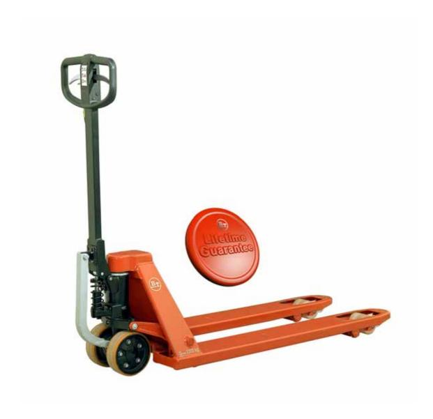
To get a hand pallet truck moving is the heaviest part of the transport. With BT Pro Lifter the truck will take the first steps by itself. A hand pallet truck loaded with 2300 kg needs a starting force of 45 kg to get into motion. With BT Pro Lifter that amount is reduced to 15 kg.
