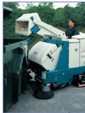
Self-sensing "smart-hopper" holds 300 lb/136 kg of debris and dumps level up to 5 ft/1530 mm.
