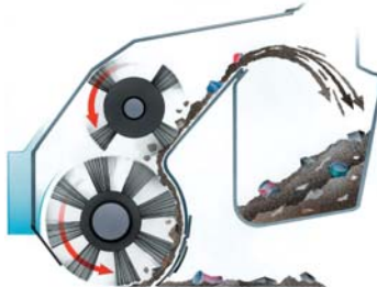
Patented, MTS system sweeps debris into the front of the hopper without brush carry-over, increasing performance and maximizing hopper space.
