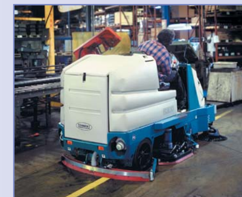
With a 45 inch/1140 mm-wide frame, the 8300 cleans the most congested manufacturing plants.
